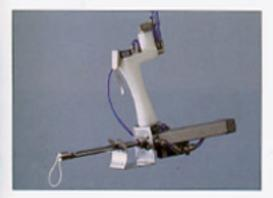
Pneumatic rib puller, a little faster, but a slightly harder work procedure.
