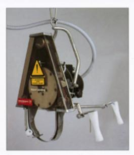
First-class safety equipment. Two-handed control with activating switch in both handles. Start protection on guard and motor brake.
