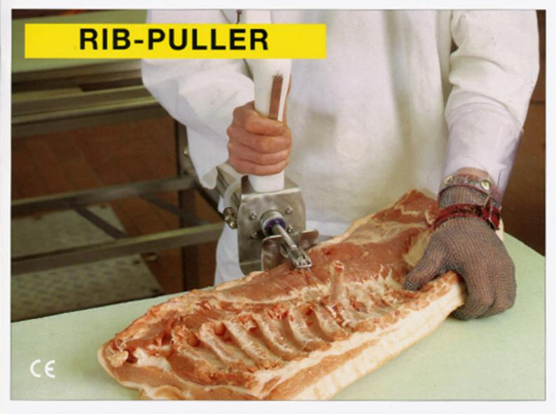
The rib puller has become an essential tool for the abattoirs where it has been introduced in production. It is used in Denmark, the UK, Sweden and Canada.
